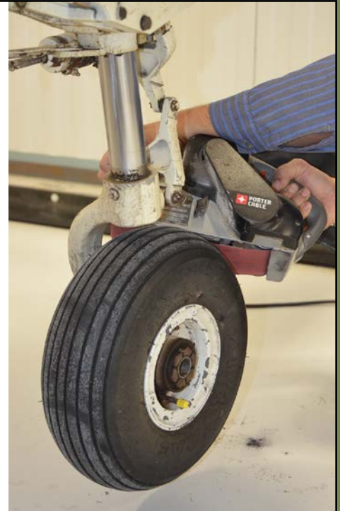
Use a belt sander to remove the shimmy wear pattern in the tread.
