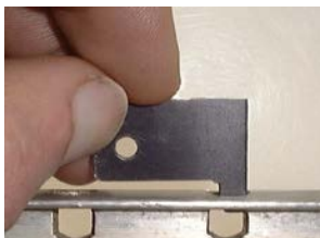
1. Place the gauge into each hole location showing wear.
