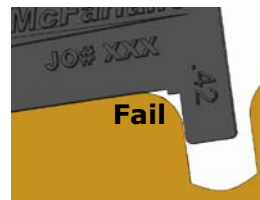
3. If the step touches the rail, lifting the gauge up, the wear is less than 0.42. If the step does not touch the rail, the wear is more than 0.42 and the seat rail must be replaced.
