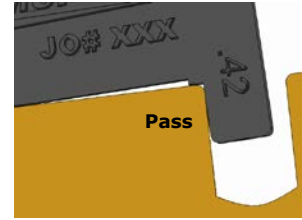
3. If the step touches the rail, lifting the gauge up, the wear is less than 0.42. If the step does not touch the rail, the wear is more than 0.42 and the seat rail must be replaced.
